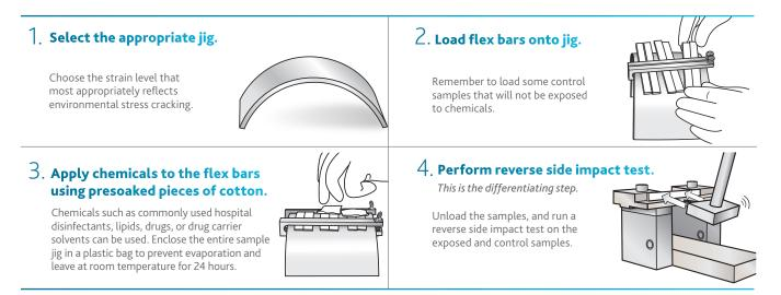
NOTE: Part and tool design and processing can affect compatibility with disinfectants; therefore, all parts and assemblies should be tested in their final form.
